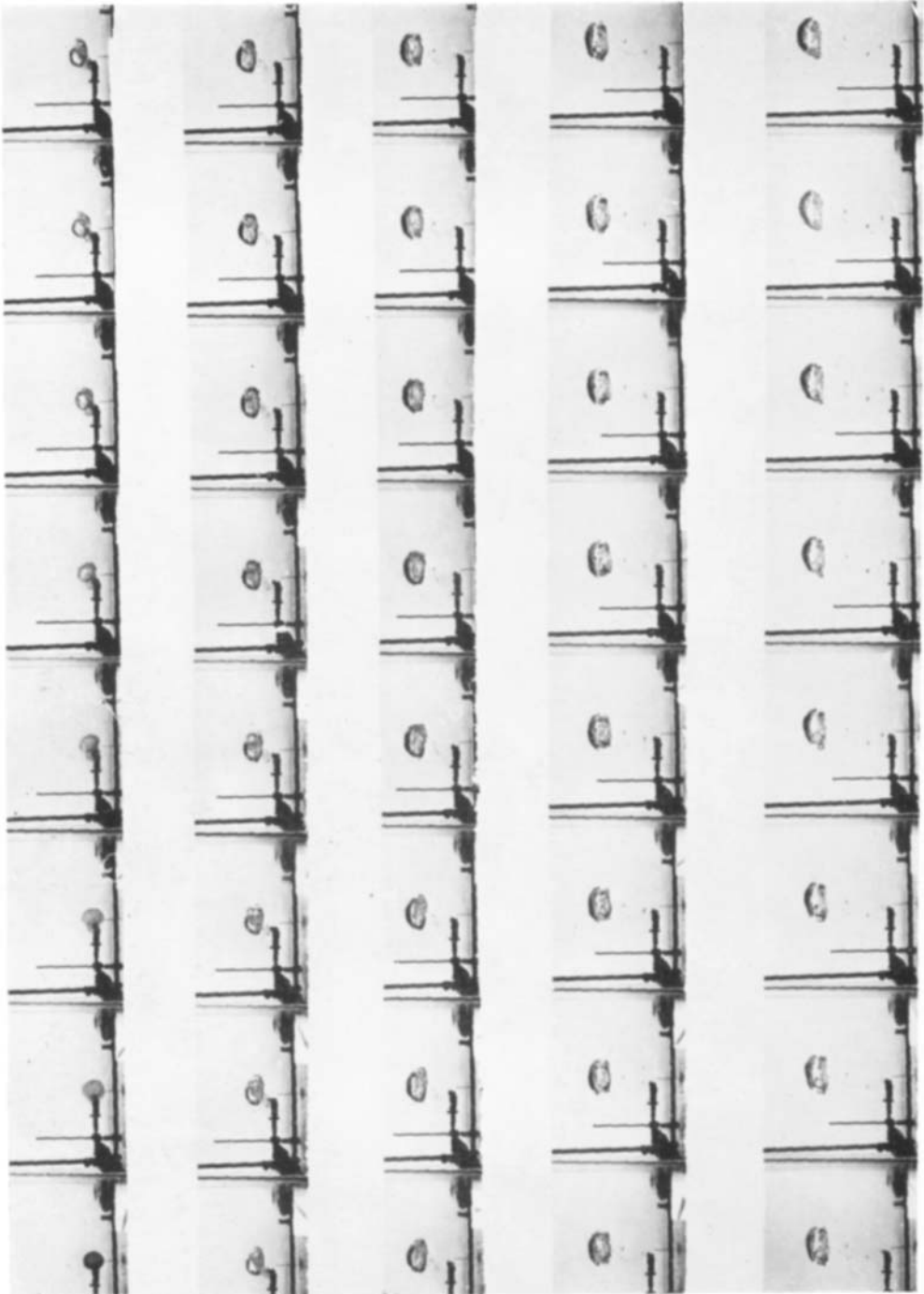
FIGURE 2. Ciné pictures at about 80 frames/sec of the initial motion of a 100 ml bubble.
